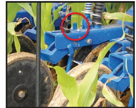
**3-WAY TOOL:** The upright tube on top of the planter unit would allow shallower placement of another seed after the disk opener passes.
