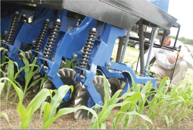
Wavy coulters cut narrow strip zones between 30-inch corn rows as seeds are dispersed through tubes onto three rows of freshly tilled soil. Different types of coulters are used depending on soil hardness.
