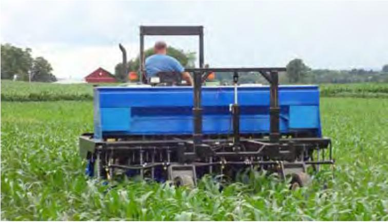
The new InterSeeder™ from InterSeeder Technologies of Woodward, Pa., simultaneously plants three rows of cover crops while spraying post-emergent herbicide and nitrogen fertilizer in single passes between four or six rows of knee-high corn. InterSeeder Technologies markets the machine under a license agreement with Penn State University.
