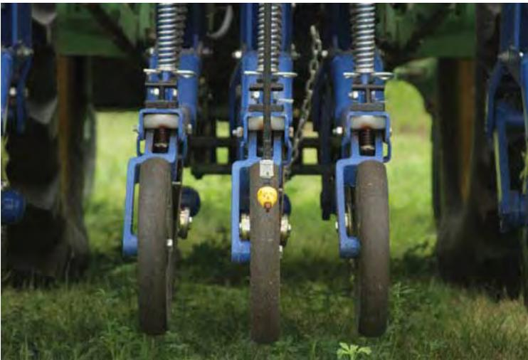
Cultipacking wheels establish troughs that embed seeds to one-half to three-quarter inch depths depending on cover crop species. InterSeeder™ all-in-one operations take place in June when corn is at V8 or less growth stage, about 18 inches high with six to eight leaves
