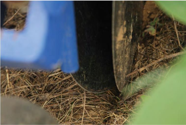
Double disk furrow openers ensure uniform seed trenches in diverse field conditions.
