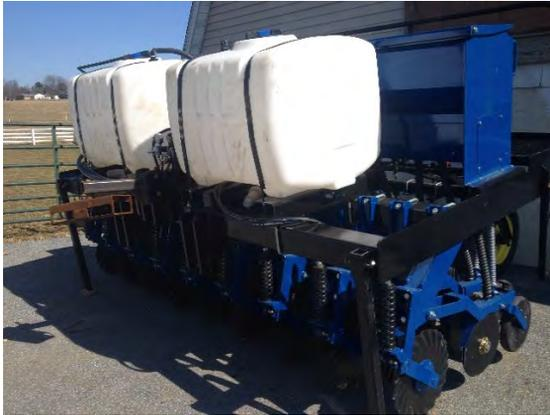
Herbicide and nitrogen tanks mounted on InterSeeder™ attach to hoses with four drop nozzles for applications shrouded by corn canopy. High pressure UAN nozzles apply nitrogen fertilizers four inches off the corn rows and four inches above the soil in a three-quarter-inch band to avoid damaging corn or cover crop.
