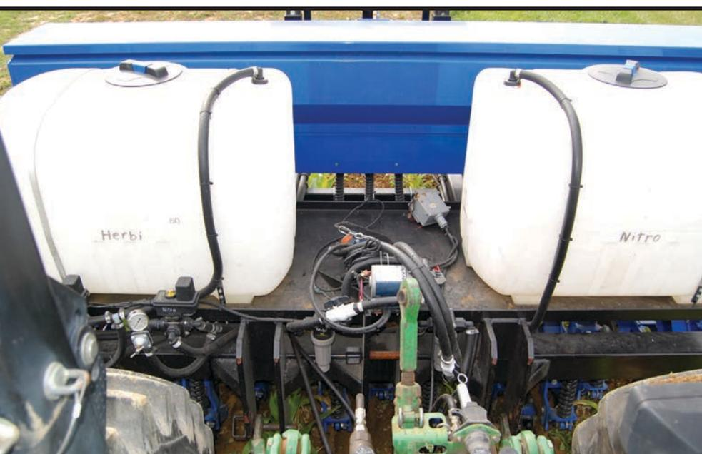
**3-POINT-HITCHED TO FLOW:** Front-mounted nitrogen and herbicide tanks are powered by a PTO pump and electric pump, respectively.
