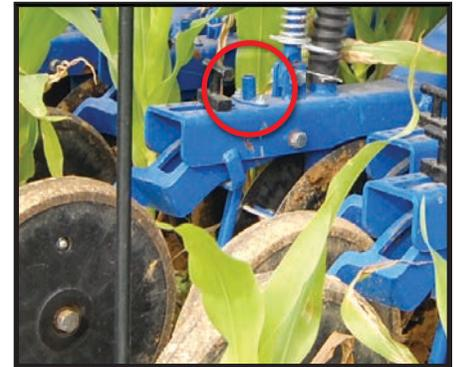
**3-WAY TOOL:** The upright tube on top of the planter unit would allow shallower placement of another seed after the disk opener passes.
